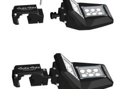
Step 1 | Remove bolt from clamp and insert ball pivot into clamp.
