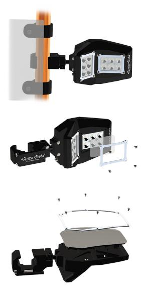
**Do you have a windshield?** | No problem! If installing our Spectrum lights/mirrors on a vehicle with a windshield, simply rotate clamp 180° and install on backside of cage. All other steps are the same.
