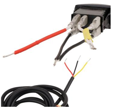
**Note** | Wires for Spectrum switch/wiring harness Yellow wire (+12v) = Constant power Black wire = Ground Red wire = Trigger (or switch) power
